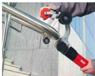
Pipe bends, sanding and polishing can be done in a clear-cut and rapid manner.
