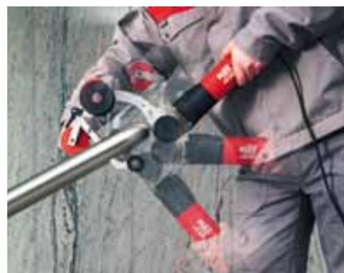
The FLEX sanding boa for the complete seamless working of tubes.
